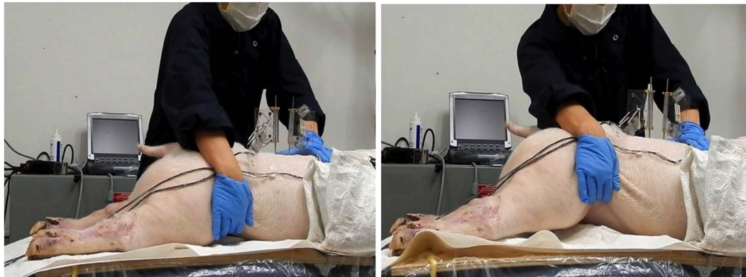
Figure 4. Passive left axial rotation movement performed by manually stabilizing L3 and manually rotating the pelvis to the left side.
