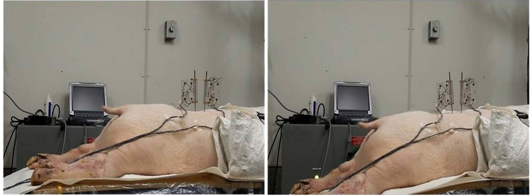
Figure 2. Passive flexion movement performed by the automatic flexion movement of the flexion-extension table.
