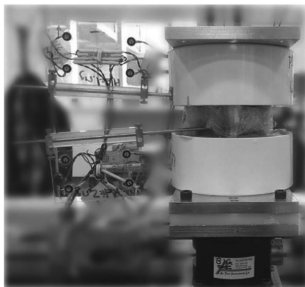
Fig 2. Potted spinal segment with L4 mounted to the 6-axis load cell and L3 fixed to a stationary cross beam.
