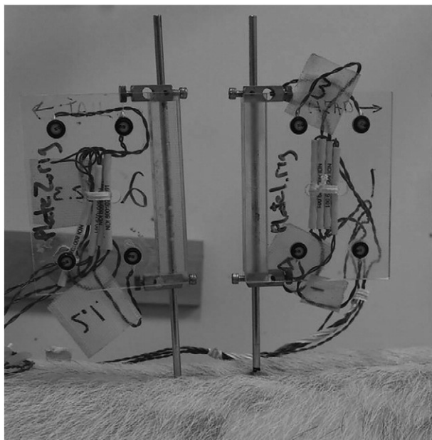
Fig 1. Rectangular flags with 4 infrared light-emitting diode markers attached to bone pins drilled into L3 and L4 vertebrae.
